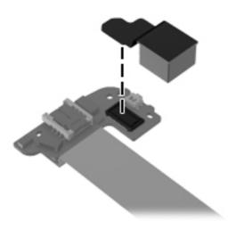
2. To remove the rear-facing webcam, turn the system board upside down, with the webcam toward you.
